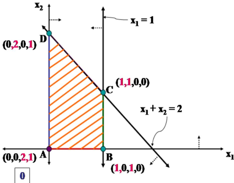
$$\left( \begin{array}{cccc|c} x_1 & x_2 & x_3 & x_4 & \text{RHS} \\ \hline 1 & 1 & 1 & 0 & 2 \\ 1 & 0 & 0 & 1 & 1 \\ \hline -3 & -1 & 0 & 0 & 0 \end{array} \right)$$
