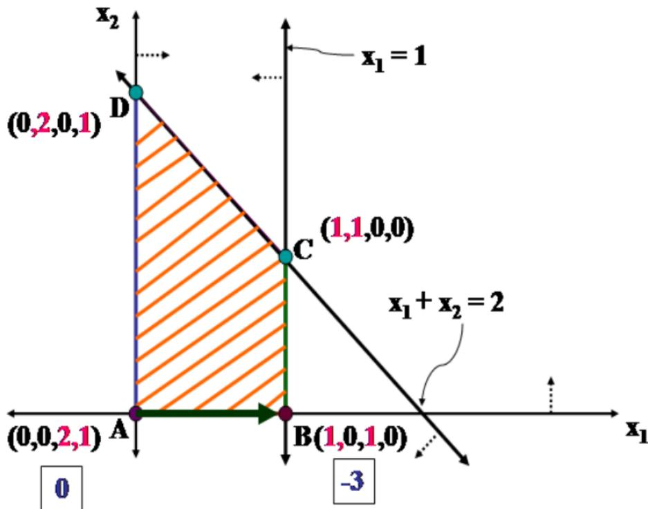
$$\left( \begin{array}{cccc|c} \mathbf{x_1} & x_2 & \mathbf{x_3} & x_4 & \mathbf{RHS} \\ \hline 0 & 1 & 1 & -1 & 1 \\ 1 & 0 & 0 & 1 & 1 \\ \hline 0 & -1 & 0 & 3 & 3 \end{array} \right)$$
