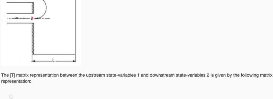
$\left\{ \begin{array}{c} p_1 \\ v_1 \end{array} \right\} = \left[ \begin{array}{cc} 1 & 0 \\ \frac{1}{-jY_{chamber} \cot k_0 L} & 1 \end{array} \right] \left\{ \begin{array}{c} p_2 \\ v_2 \end{array} \right\}$
