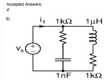
In the circuit above,  $v_s(t) = 4\sin(10^6t)$  V. In steady state  $i_1 = I_p\cos(\omega t + \phi)$ . Determine  $V_p$  and  $\phi$ .
