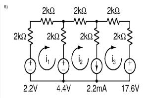
Setup the mesh analysis equations for the circuit above with the given source vector. The format of the equations is as shown.
