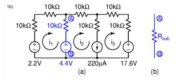
In the circuit above, the entire combination between A and B, shown in blue, must be substituted by a resistance of value  $R_{sub}$  as shown in (b). Determine  $R_{sub}$ . You can use any method you wish, but you are encouraged to use mesh analysis. You could also possibly use part of the solution to one of the previous problems.
