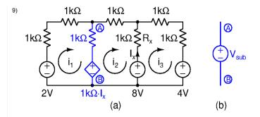
In the circuit above, the entire combination between A and B, shown in blue, must be substituted by a voltage source of value  $V_{sub}$  as shown in (b). Determine  $V_{sub}$ . You can use any method you wish, but you are encouraged to use mesh analysis. You could also possibly use part of the solution to one of the previous problems.
