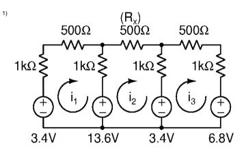
Setup the mesh analysis equations for the circuit above with the given source vector. The format of the equations is as shown.
