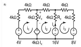
In the circuit above, determine the contribution of *only the* 4V source to  $V_x$ . You can use any method you wish, but you are encouraged to use mesh analysis. You could also possibly use part of the solution to one of the previous problems.
