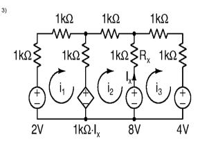
Setup the mesh analysis equations for the circuit above with the given source vector. The format of the equations is as shown.
