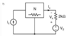
In the circuit above,  $I_x = 0.5$  mA when  $I_1 = 4$  mA,  $V_2 = 4$  V and  $V_x = 1$  V when  $I_1 = 2$  mA,  $V_2 = 8$  V. Determine the power dissipated in the 2k $\Omega$  resistor when  $I_1 = 8$  mA,  $V_2 = 16$  V. The network N consists only of resistors.
