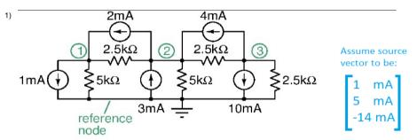
Setup the nodal analysis equations for the circuit above. Enter the G matrix in the space provided below.
