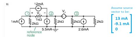
Setup the nodal analysis equations for the circuit above. Enter the G matrix in the space provided below,
