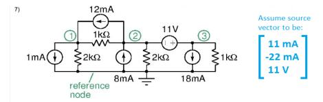
Setup the nodal analysis equations for the circuit above. Enter the G matrix in the space provided below.
