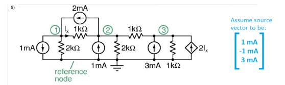
Setup the nodal analysis equations for the circuit above. Enter the G matrix in the space provided below,
