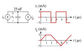
In the figure above, determine the voltage  $v_c$  at  $t=6\mu s$ . The capacitor is initially discharged (i.e. the capacitor voltage is zero at t=0). (The waveform consists
