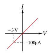
A resistor's *I-V* characteristics are shown in the figure above. Determine its resistance.
