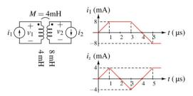
In the figure above, determine the voltage  $v_2$  at  $t=4\mu s$ . (The waveform consists of straight line segments)
