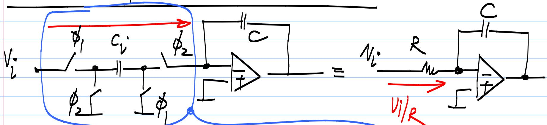
In each cycle ( $\approx T_s$ ), a charge  $C_i V_i$  is transferred to  $C$
