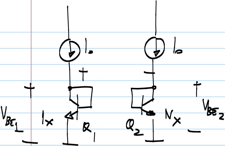
$V_{BE_1} - V_{BE_2}$  must appear across a resistor (must have zero  $T_C$ )
