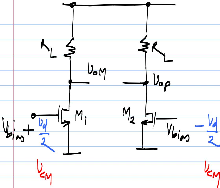
$$A_D = \frac{V_{op} - V_{oM}}{V_d} = g_m \cdot R_L$$
