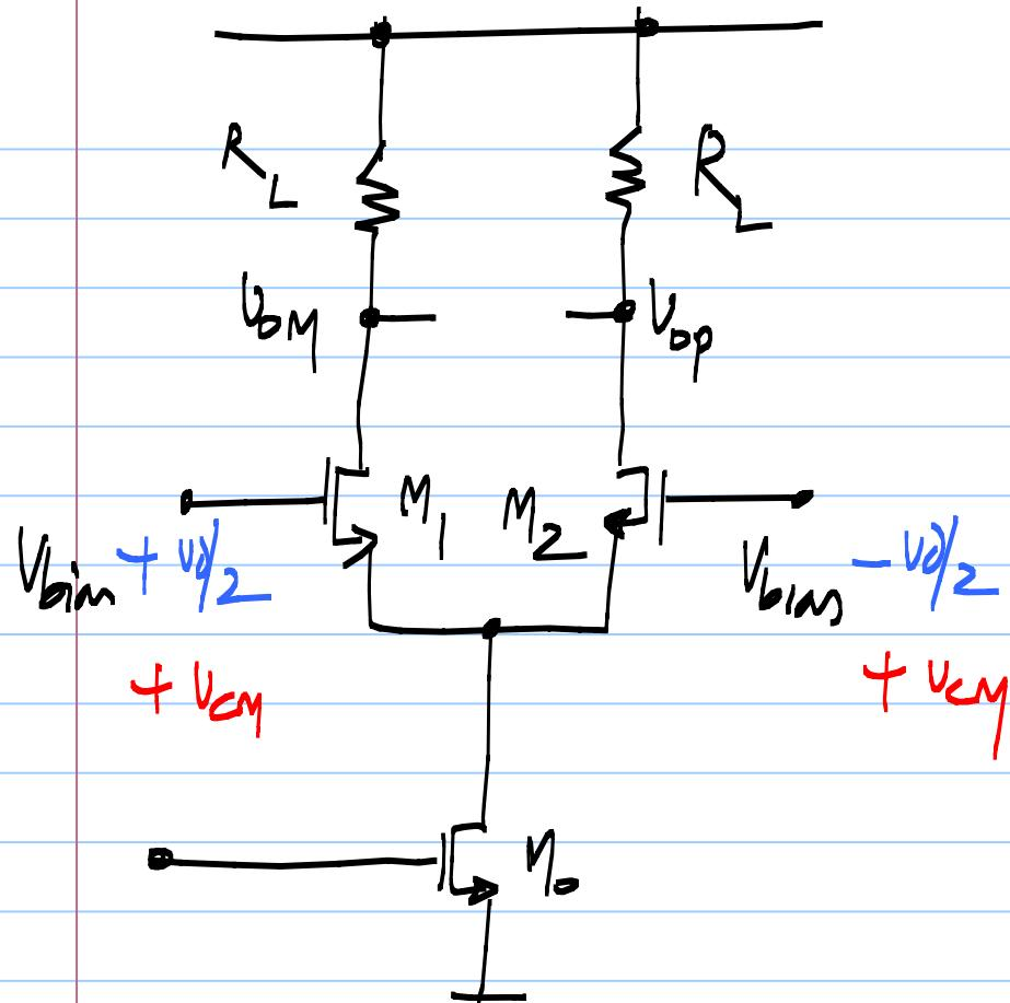
$$A_d = \frac{V_{op} - V_{oM}}{V_d} = g_m \cdot R_L$$
