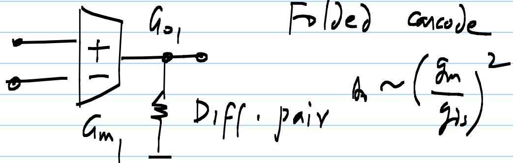
$$\left( \frac{g_m}{g_{D_s}} \right)^2 \left( \frac{g_{m11}}{g_{D_{s1}} + g_{D_{s2}} + g_{L2}} \right)$$
