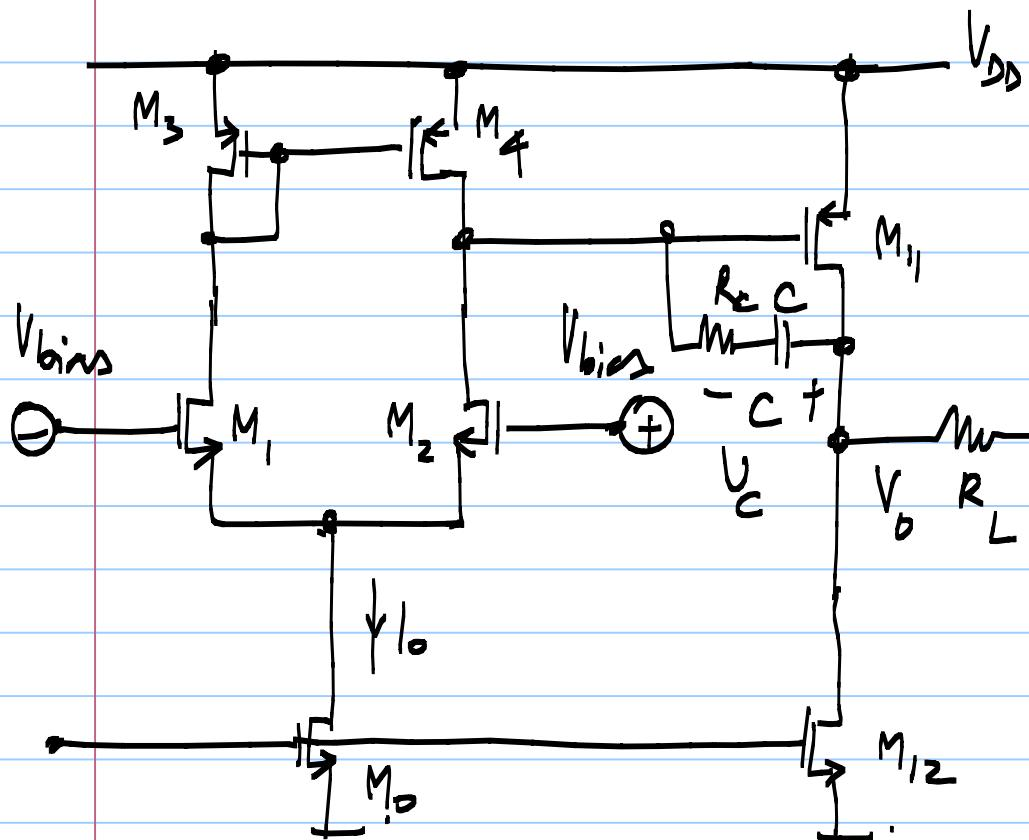
$$\left[ \begin{array}{l} V_{T_1} + V_{DSAT_1} < V_{bias} < V_{DD} - V_{SG3} + V_{T_1} \\ + V_{DSAT_0} \end{array} \right]$$
