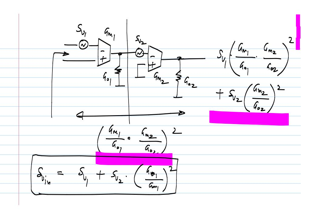
$$S_{v_{in}} \simeq \frac{16}{3} \cdot \frac{kT}{g_{m_i}} \left(1 + \frac{g_{m_3}}{g_{m_i}}\right)$$
