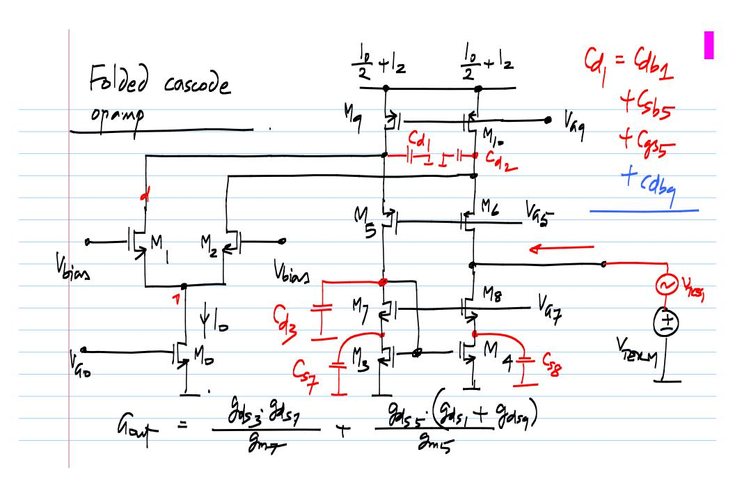
cascode transconductor parasitic capacitances
