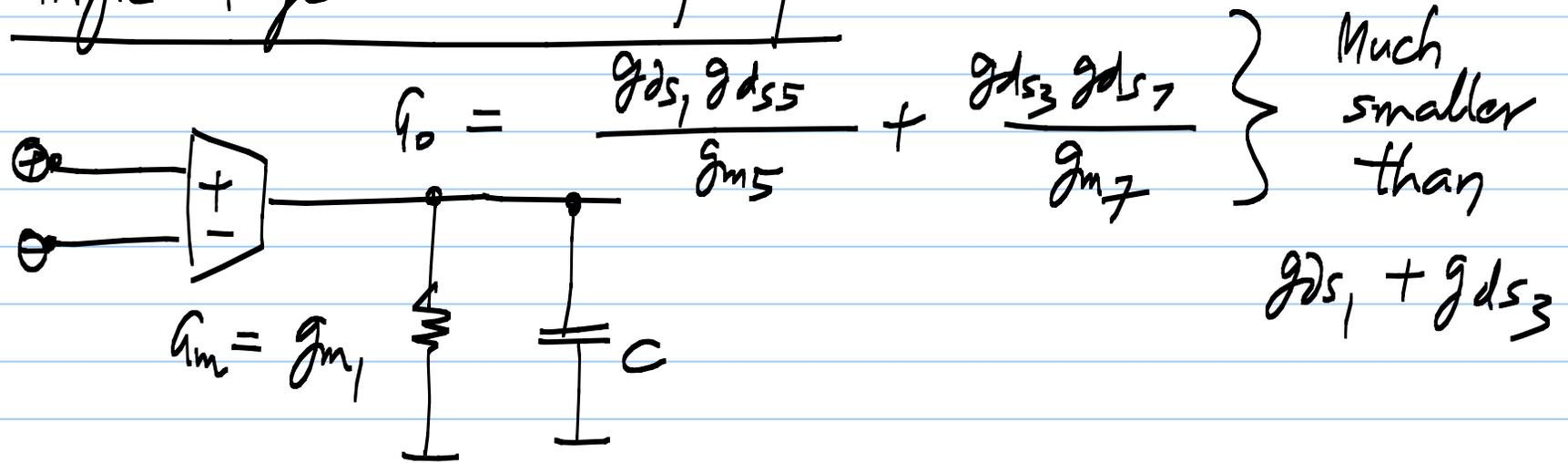
$$\frac{g_{m1}}{g_{ds1} + g_{ds3}} \sim \left( \frac{g_m}{g_{ds}} \right); \quad \frac{g_{m1}}{\frac{g_{ds1} g_{ds5}}{g_{m5}} + \frac{g_{ds3} g_{ds7}}{g_{m7}}} \sim \left( \frac{g_m}{g_{ds}} \right)^2$$
