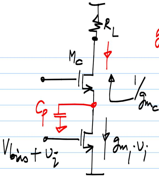
$$g_{m_i} \cdot v_i(s) \frac{g_{m_c}}{g_{m_c} + sC_p} = g_{m_i} \cdot v_i(s) \cdot \frac{1}{1 + \frac{sC_p}{g_{m_c}}}$$
