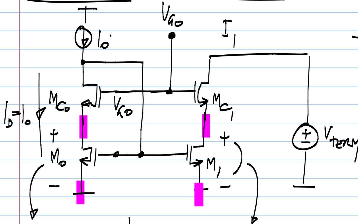
$$\Delta V_{TERM} = g_{mC} \cdot g_{m1}^{-1}$$
