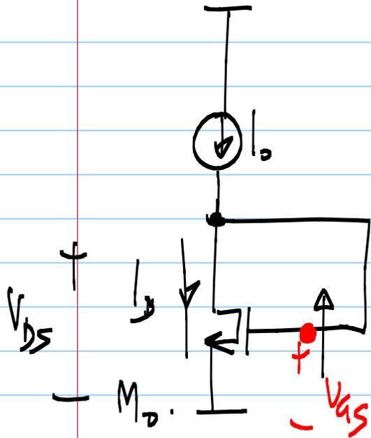
$$V_{DS0} = V_{GS0}$$
