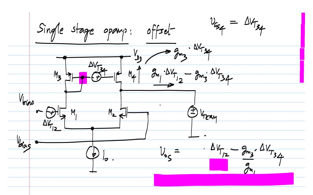
$$\frac{1}{V_{05}} = \frac{1}{V_{72}} + \left(\frac{9m_3}{9m_1}\right)^2 \cdot \frac{1}{V_{734}}$$
