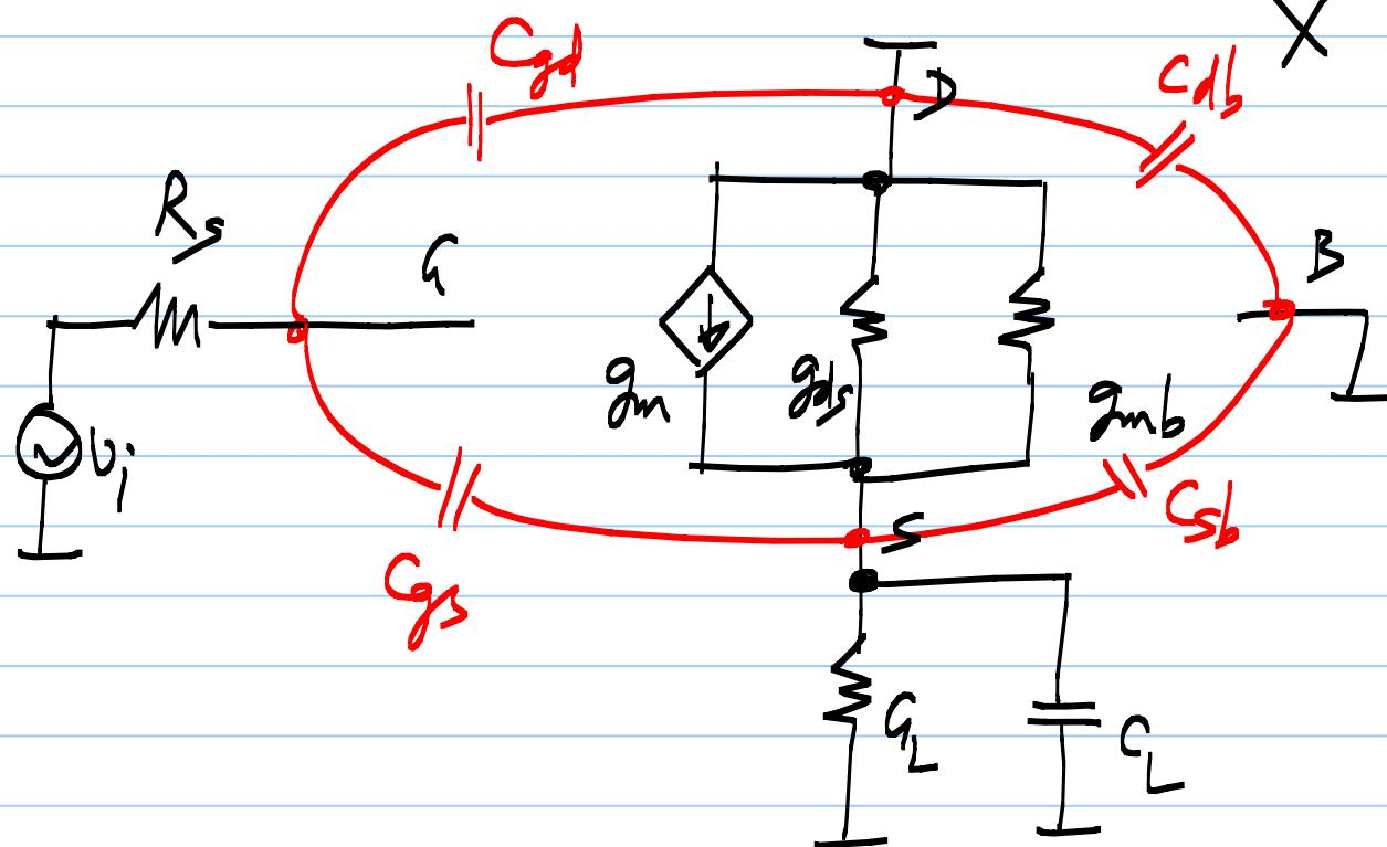
$$C_L' = C_{sb} + C_L$$
