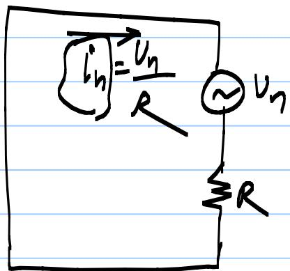
Spectral density of  $i_n, v_n$  {noise in a resistor  $R$ }
