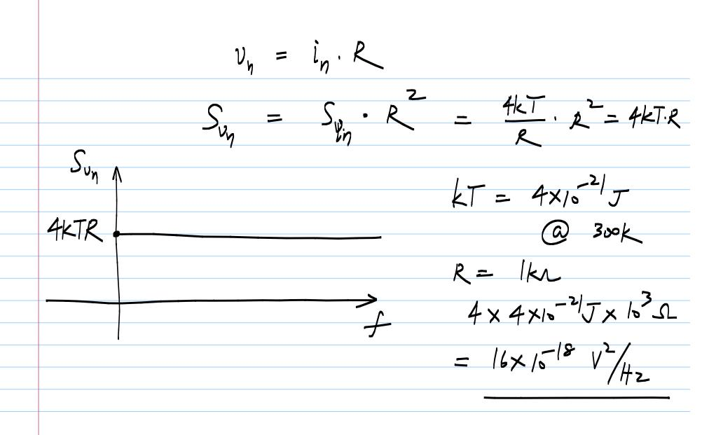
$$S_{i} = \frac{4kT}{R} \quad A^{2}/H_{2} \quad S_{i} = \frac{4kT \cdot R}{H_{2}} \quad \frac{V^{2}}{H_{2}}$$
