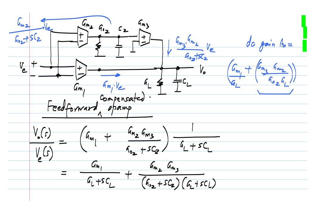
$$\frac{V_{s}(s)}{V_{e}(s)} = \frac{G_{m_{1}} + \frac{G_{m_{2}}G_{m_{3}}}{K_{o_{2}} + sC_{2}} \frac{1}{G_{L} + sC_{L}}}{G_{L} + sC_{L}}$$
