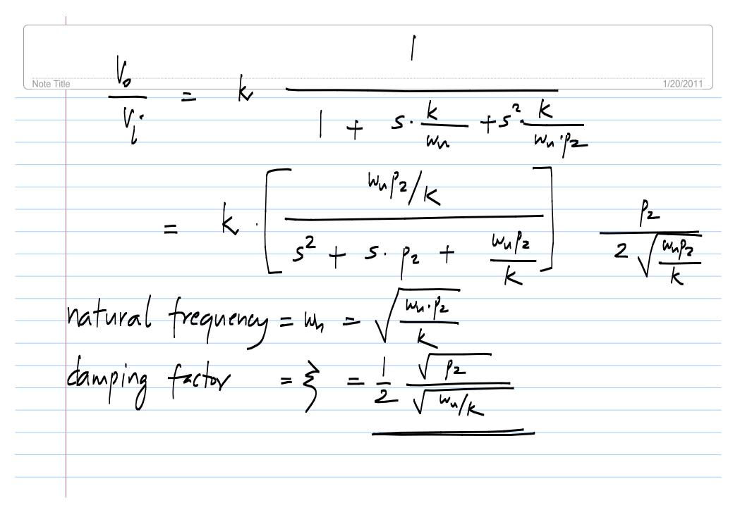
Negative feedback amplifier with on extra pole in the fird path Note Title 1/20/2011 dc gain = Second order transfer fn. Nn 3~~] 1 Desired rosponse -ical danj critically damped ; 1.0 underdamped
