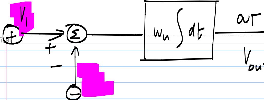
$$V_{\text{out}} = w_n \int (V_1 - V_2) dt$$
