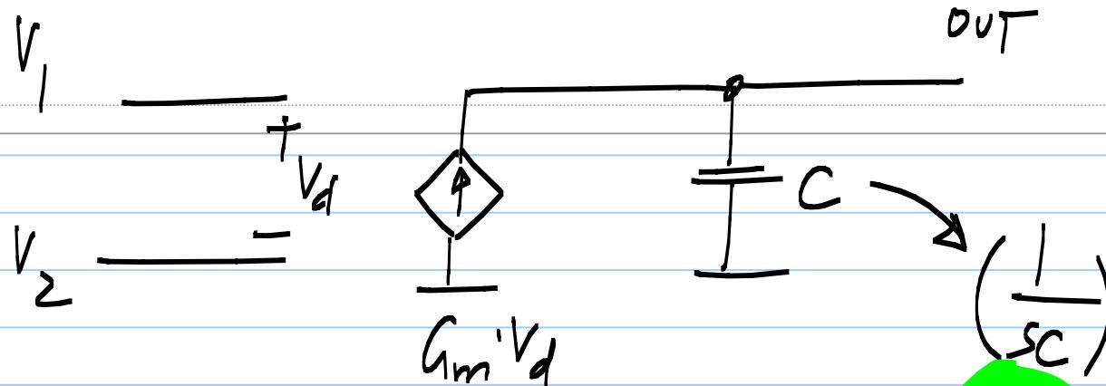
$$V_{\text{out}} = G_m \cdot V_d \cdot \frac{1}{sC} = \frac{G_m}{sC} (V_1 - V_2)$$
