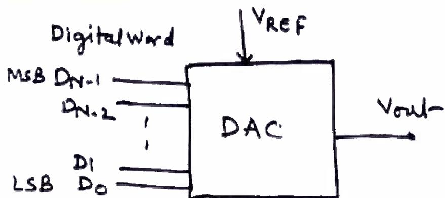
Typically, the output of DAC is a fraction  $F$  of  $V_{REF}$ .
