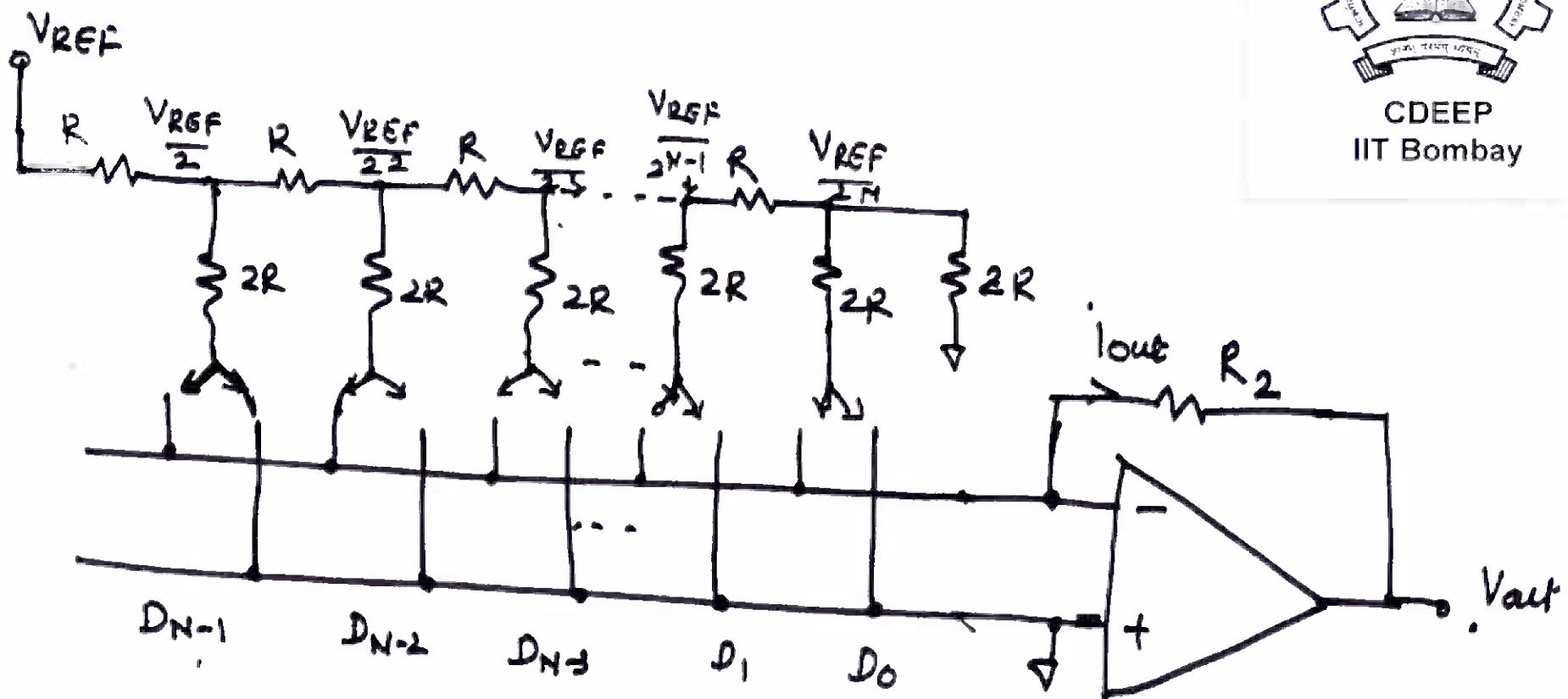
$$V_o = -i_{out} R_2, \quad i_{out} = \sum_{k=0}^{N-1} D_k \cdot \frac{V_{REF}}{2^{N-k}} \cdot \frac{1}{2R}$$
