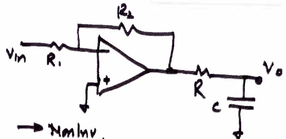
$$\frac{V_o}{V_{in}} = -\left(\frac{R_2}{R_1}\right) \cdot \frac{1}{1+s/(C/R)}$$
