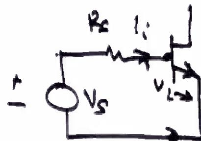
Output Circuit: Set  $V_o = 0$  (current sampling) &  $i_i = 0$  (voltage sampling)
