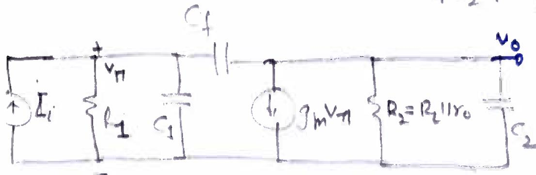
$$= \frac{g_m}{\frac{C_1 C_2}{C_f} + (g_m + C_2)}$$
