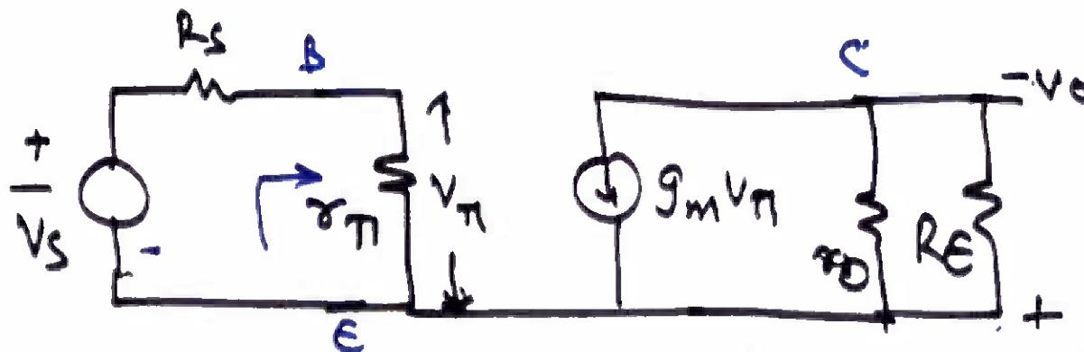
$$\therefore A_{OL} = \frac{V_o}{V_s} = + \frac{r_\pi}{r_\pi + R_s} \cdot g_m R_E$$
