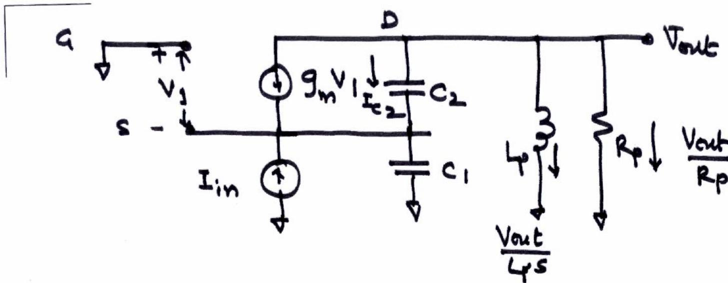
$$\therefore V_1 = - \left( I_{in} - \frac{V_{out}}{L_p s} - \frac{V_{out}}{R_p} \right) \cdot \frac{1}{C_1 s}$$
