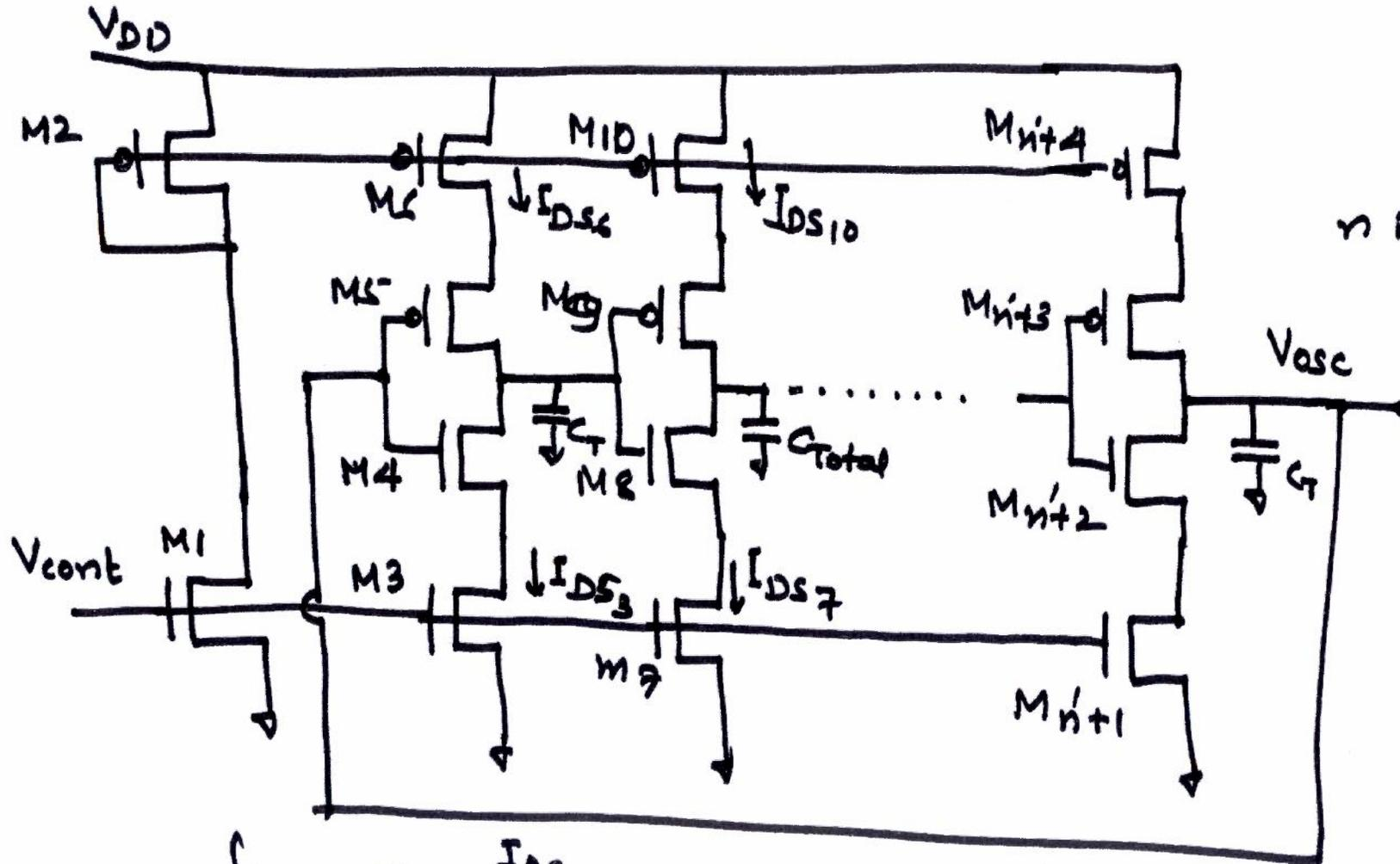
$$f_{osc} = \frac{I_{DS}}{N \cdot C_{Total} \cdot V_{DD}}$$
