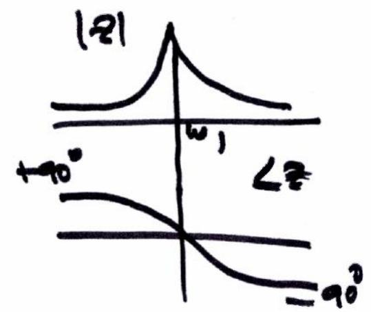
In ideal LC circuit at oscillation frequency the  $Z_{TC}$  (i.e. for Tuned Circuit) is infinite.
