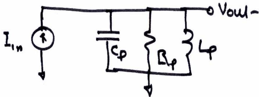
Oscillations die as  $R_p$  dissipates power
