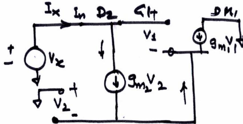
$$I_x = g_{m2} V_2 = -g_{m1} V_1$$
