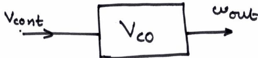
$$\omega_{\text{out}} = \omega_0 + K_{\text{VCO}} \cdot V_{\text{cont}}$$
