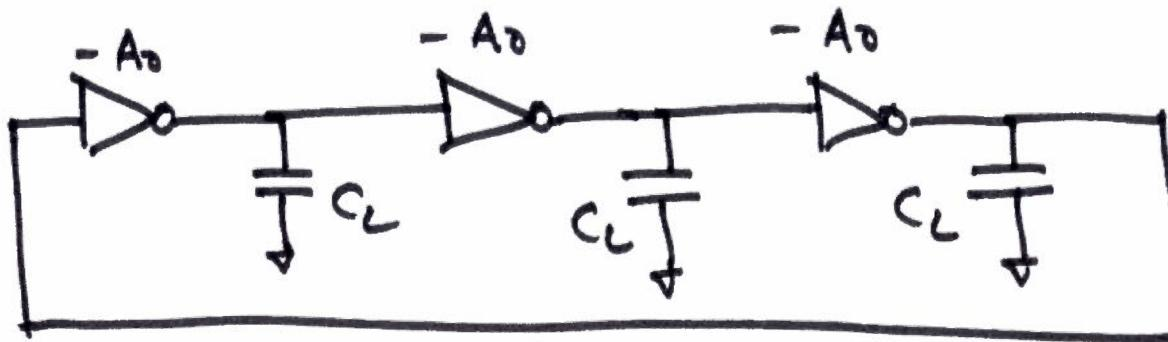
Here  $\omega_0 = (\gamma_{out} \cdot C_L)^{-1}$ ;  $A_0$  is a Stage Gain
