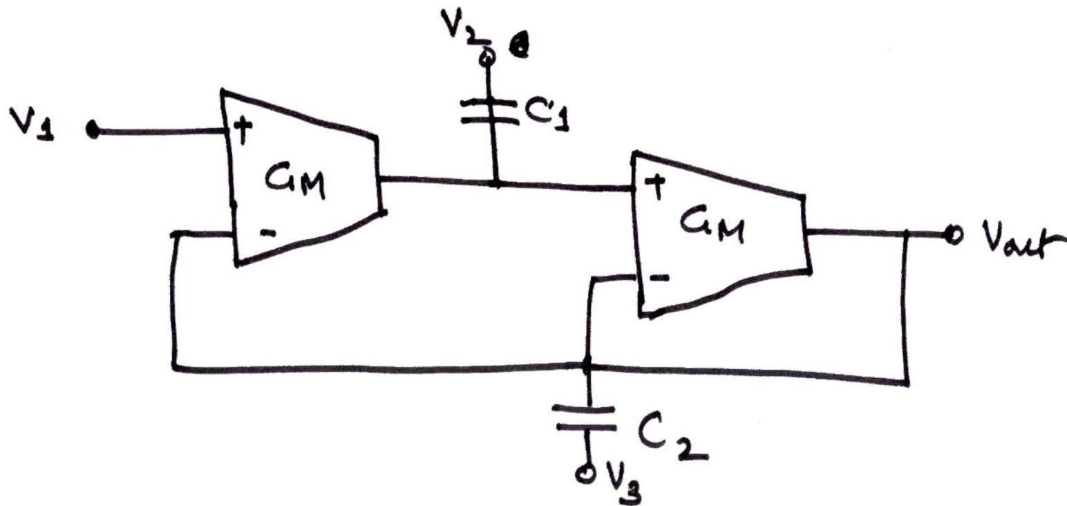
If we put  $V_2$  and  $V_3$  to Ground, we get -
