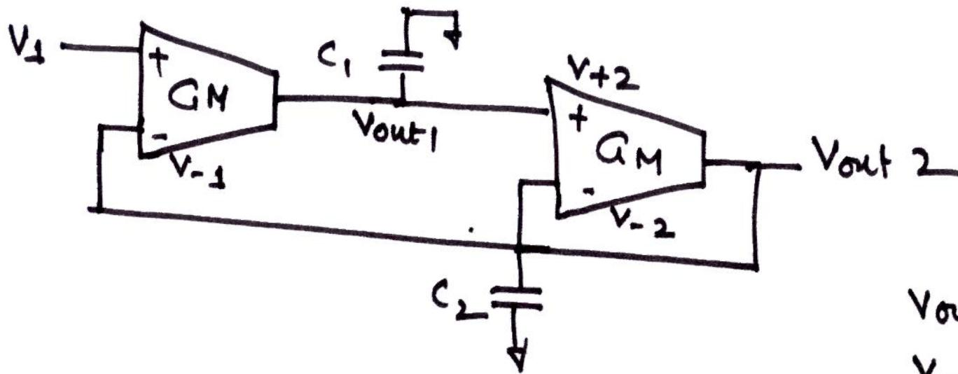
$$V_{out1} = G_M (V_1 - V_{-1}) \cdot \frac{1}{j\omega C_1}$$
