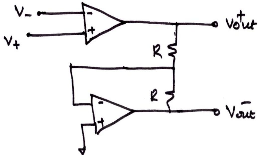
Due to difference in Input connectivity in two OPAMPS, the Phase Margins for two Differs a lot and hence Bandwidth observed for this case is very much Limited.
