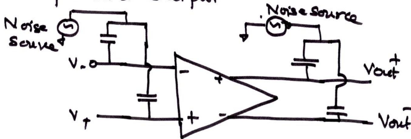
$$V'_- = V_- + V_N \quad , \quad V'_+ = V_+ + V_N$$
