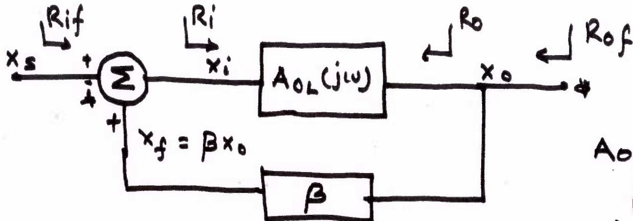
$A_{OL}(j\omega)$  = Open Loop Gain $\beta$  = Feedback factor $A_{CL}(j\omega)$  = Closed Loop Gain
