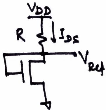
$$\text{Clearly } V_{DS} = V_{ref}$$
