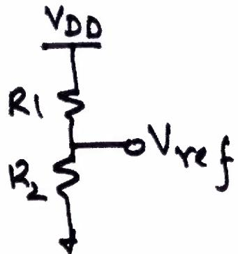
$$V_{ref} = \frac{R_2}{R_1 + R_2} V_{DD} = \frac{1}{1 + \frac{R_1}{R_2}} V_{DD}$$
