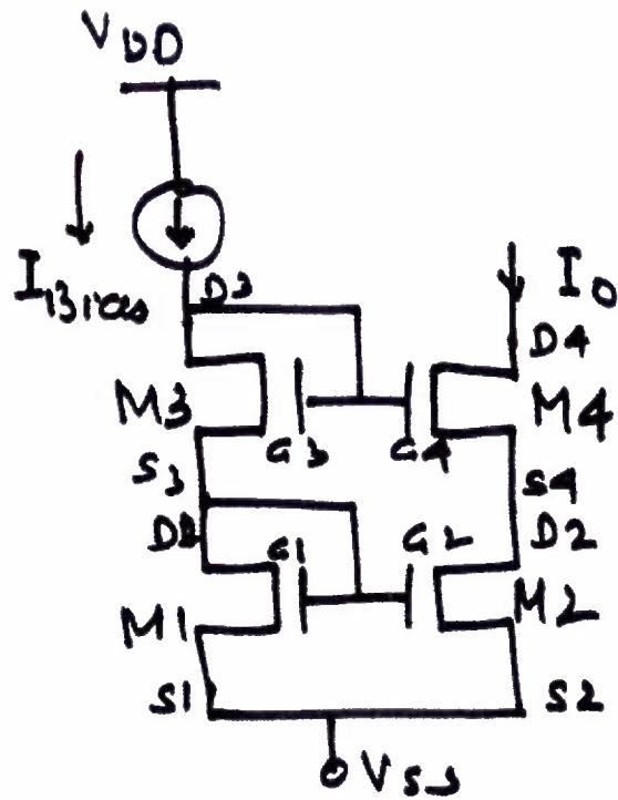
M<sub>2</sub> & M<sub>4</sub> form Cascode Stage leading to Higher Rout.
