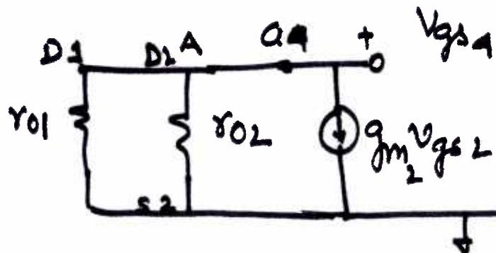
$$V_{sb4} = V_{gs2} = V_{gs3} = I_x (r_{o3} \parallel \frac{1}{g_m3})$$
