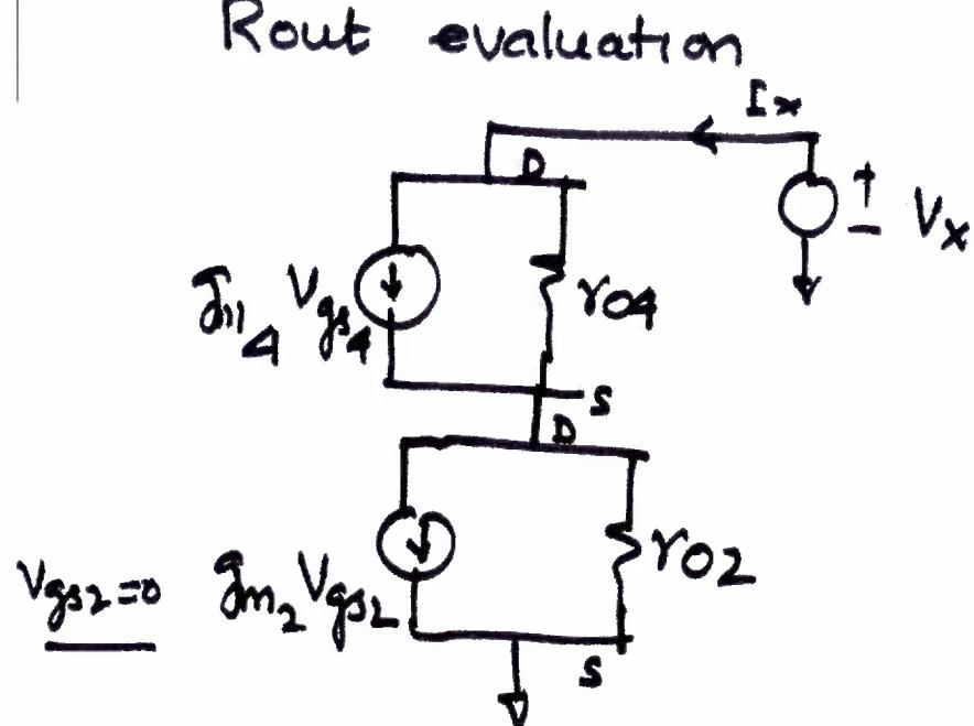
$$R_{out} = r_{04} (1 + g_m r_{02}) + r_{02}$$
