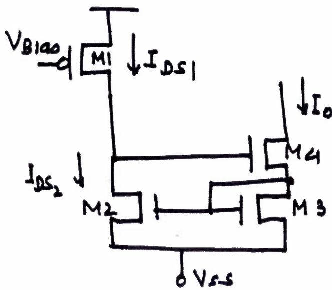
By Using P-device with proper bias we can create stable & Reference current  $I_{DS1}$ .  $V_{BIASO}$  is normally taken from a 'stable Band Gap reference'
