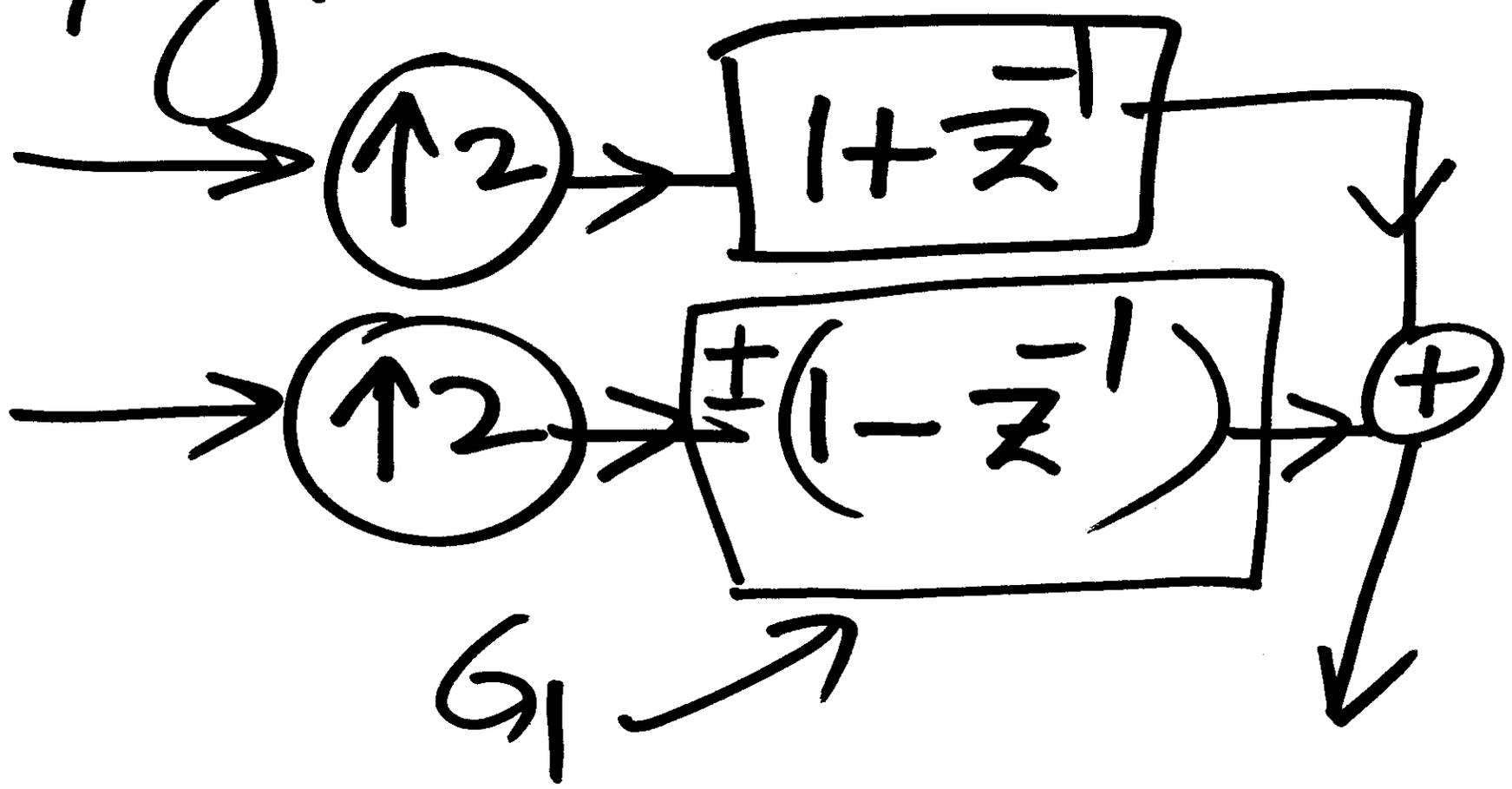
$$\tau_1(z) = \left. \begin{aligned} & \frac{1}{2} \{ G_0(z) H_0(-z) \\ & + G_1(z) H_1(-z) \} \end{aligned} \right\}$$
