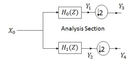
$H_0(Z)$  is a low pass filter with a cut off frequency  $\frac{\pi}{2}$  and  $H_1(Z)$  is a high pass filter with a cut off frequency  $\frac{\pi}{2}$ . Analysis section analyzes or breaks down the input in two components.
