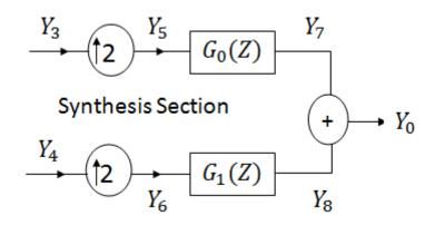
$G_0(Z)$  is a low pass filter with a cut off frequency  $\frac{\pi}{2}$  and  $G_1(Z)$  is a high pass filter with a cut off frequency  $\frac{\pi}{2}$ . Synthesis section re-synthesize output from the inputs.
