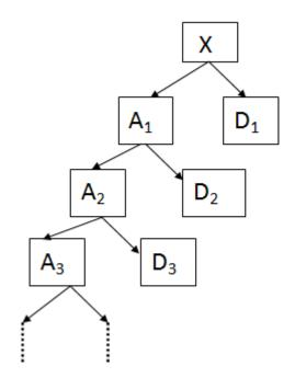
This is trend and surprise abstraction tree (TSA tree). Here 'X' is original sequence, 'A' and 'D' are are Discrete wavelet transform of the parent node (X).
