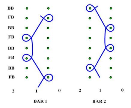
Apparently the guide bar 1 wraps yarn around needles of front bed only while the guide bar 2 wraps yarn around needles of back bed. Hence two separate fabric layers can apparently be created by the two beds. However no fabric can eventually form as there is no yarn connecting the two layers of fabric expected to be formed on the front and back beds. In the absence of holding down sinkers, such connections are necessary to hold the fabric down during the upward journey of needles of one bed
