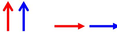
Figure 3.3: Schematic drawing of broadside and head-to-tail configurations for a pair of ferromagnetically coupled magnetic moments.
