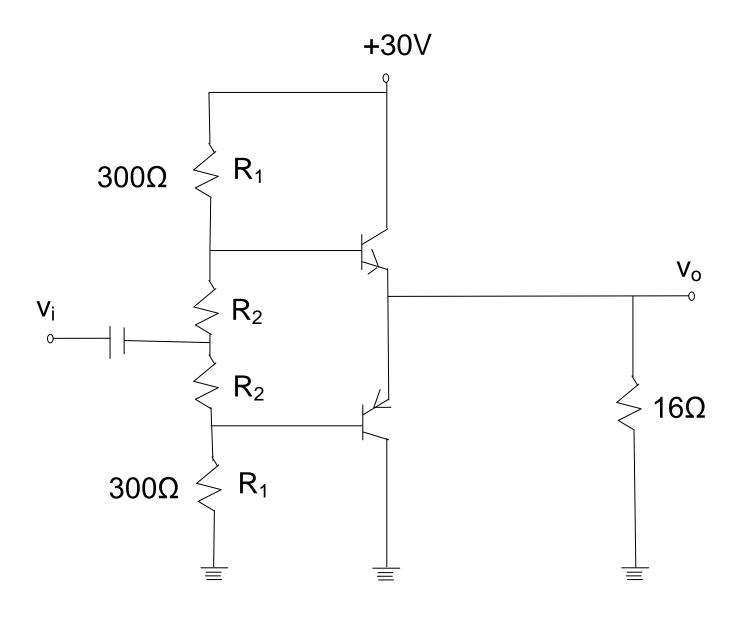
Trickle current which flows through resistors R<sub>2</sub> and produces a voltage drop of 0.7 V across base – emitter junction over comes cross – over distortion in push – pull amplifier. For analysis purposes, it is sufficient to consider only half of the circuit for reasons of symmetry, and V<sub>CC</sub> of half (= V<sub>CC</sub>/2 = 30/2 = 15V) is to be taken for one transistor.
