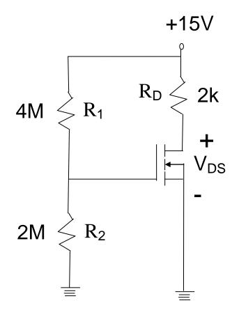
The gate current, I<sub>G</sub>, is zero in a MOSFET. Then, from voltage divider network,
