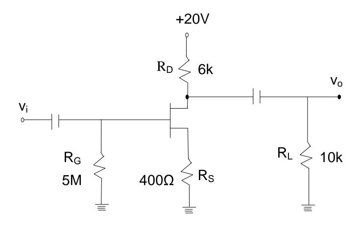
When the source resistance  $R_S$  is not by passed, the voltage gain is,
