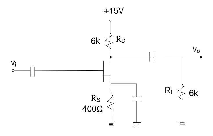
In case, the source resistance  $\mathsf{R}_\mathsf{S}$  is ac grounded as done in the circuit of fig. the gain of amplifier is,
