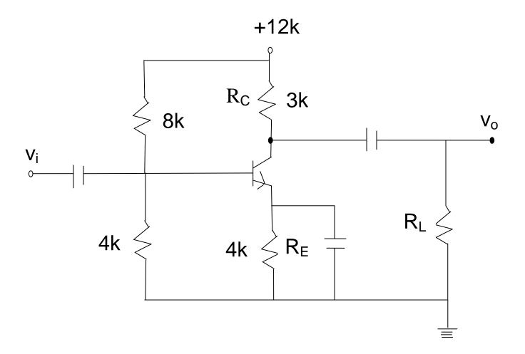
The voltage gain of the common emitter amplifier with resistor  $R_E$  by-passed (see fig.) is expressed as
