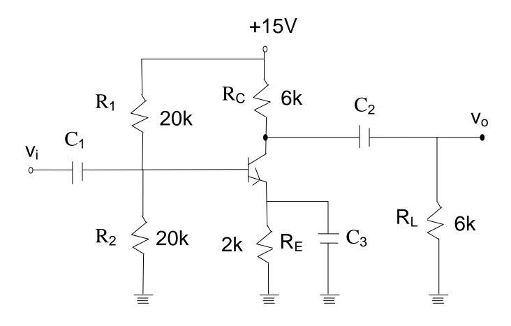
The magnitude of voltage gain with h-parameters  $h_{oe}$  and  $h_{re}$  dropped, and emitter resistance  $R_E$  by-passed by capacitor  $C_3$  is
