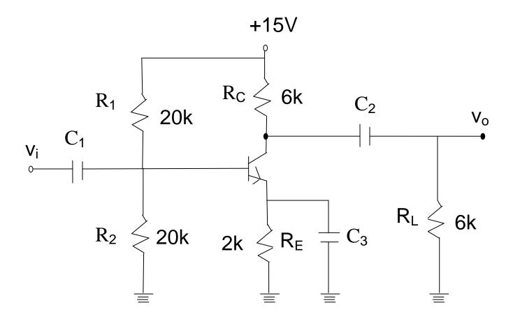
With by-pass capacitor  $C_3$  (in fig.) removed, the gain of a amplifier falls and input impedance of the amplifier increases.
