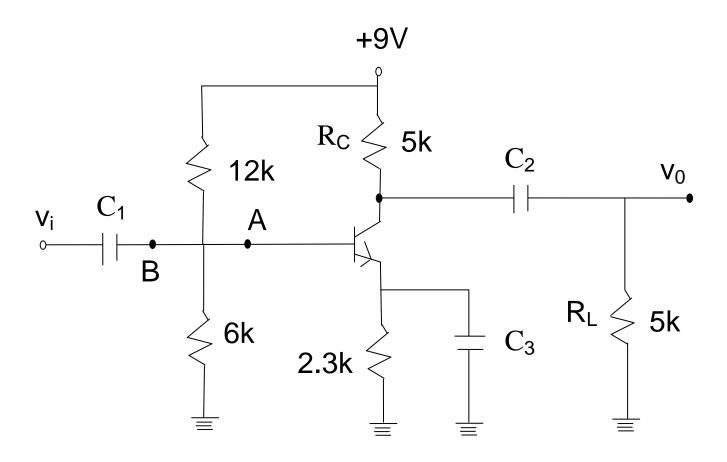
The voltage gain  $A_V$ , for a common emitter amplifier with resistor  $R_E$  by- passed is
