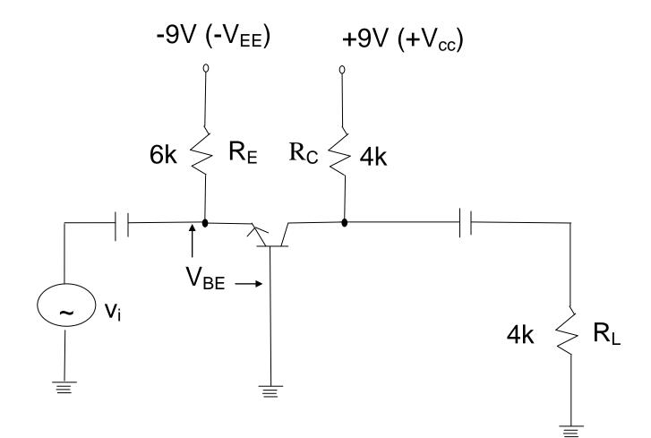
The dc voltage sources have to be grounded for ac analysis of the amplifier. Then the input impedance of the CB amplifier (in fig.) is
