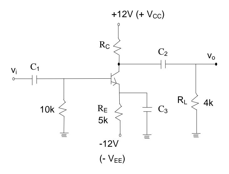
In case,  $R_E$  is by-passed, the voltage gain  $A_v$  of the amplifier is,
