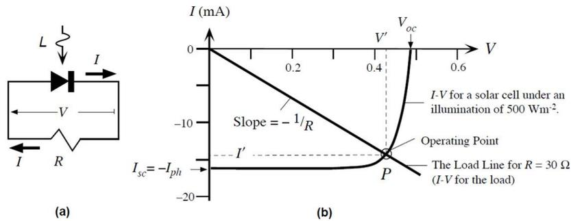
Figure 1: (a) Schematic of a solar cell equivalent circuit. (b)  $I$ - $V$  curve under illumination of  $500 \text{ Wm}^{-2}$ . Adapted from *Principles of Electronic Materials* - S.O. Kasap
