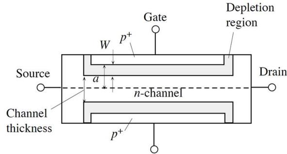
Figure 1: For problem 3. Schematic of a  $n$ -channel MOSFET. Adapted from *Principles of Electronic Materials - S.O. Kasap*
