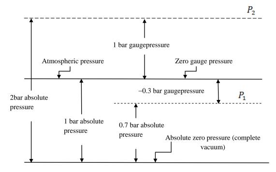
Figure 1.3 Difference between absolute and gauge pressure.
