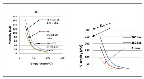
**Figure 1.10**Typical kinematic viscosities for a range of fluids. (a) Some fire-resistant fluids. (b) An ISO 32 mineral oil.
