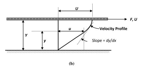
**Figure 1.8**Velocity profiles across parallel plates: (a) Linear (no bulk flow) and (b) linear (bulk flow to right).
