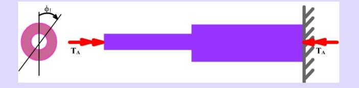
By applying  $T_A$  to the unloaded bar, as shown in the above figure, end rotation  $\theta_1$  at end A is found.
