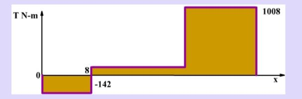
The torque diagram for the shaft is shown in the above figure. The direction of the internal torque vector T on the left part of an isolated shaft segment coincides with that of the positive x axis, it is taken as positive. Note that most of the applied torque is resisted at the end E. Since the shaft from A to C is more flexible than from C to E, only a small torque develops at A.
