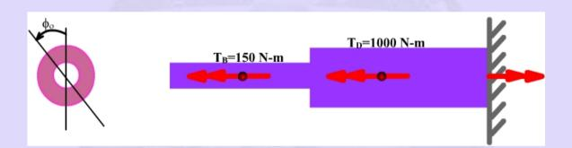
There are two unknown reactions,  $T_A$  and  $T_E$ . One of them can be considered as redundant, and, arbitrary, reaction  $T_A$  is removed. This results in the free-body diagram shown in the above figure. Then the end rotation is calculated as  $\theta_0 = 23.3 \times 10^{-3}$  rad.
