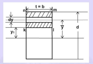
The cross sectional area of the beam is shown in the figure. A longitudinal cut through the beam at a distance  $y_1$ , from the neutral axis, isolates area klmn. (A<sub>1</sub>).
