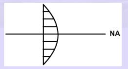
Max Shear Stress occurs at the neutral axis and this can be found by putting y = 0 in the equation 1.
