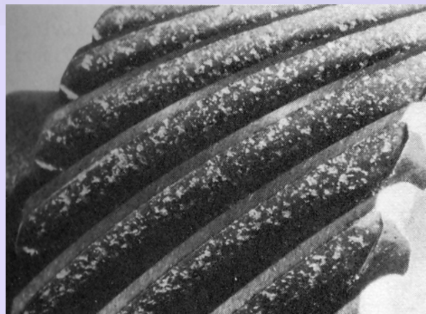
Fig. 6.6 Moderate adhesive wear
