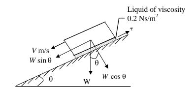
For a thin film, velocity distribution can be assumed to be linear. Hence, the velocity gradient is found to be
