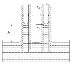
Equating the weight of water column in the annulus with the total surface tension force, we have
