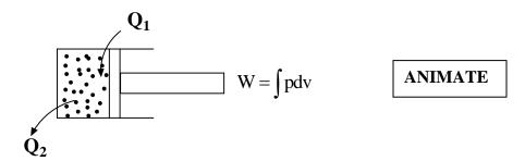
**1.1.2.1**A- Conversion of heat to mechanical energy in a piston cylinder arrangement.
