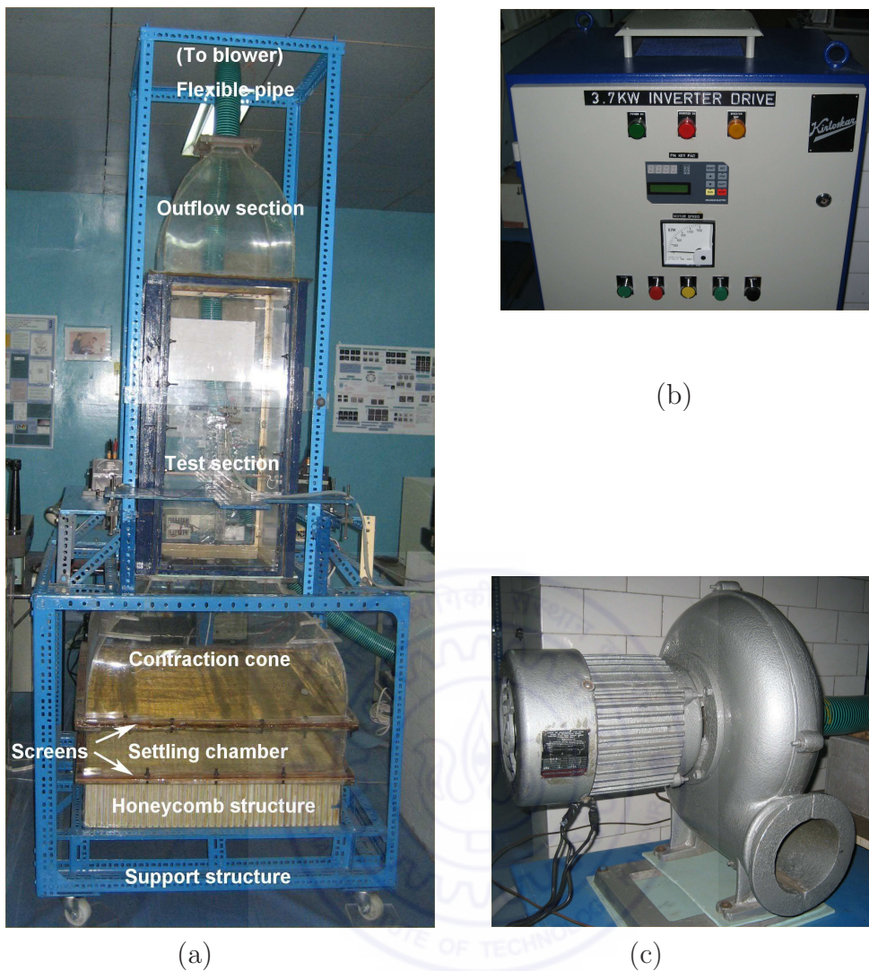
Figure 3.3: Photograph of the (a) Vertical flow facility, (b) Frequency-based inverter drive and, (c) Blower, connected through a flexible pipe at the end of the outflow section.
