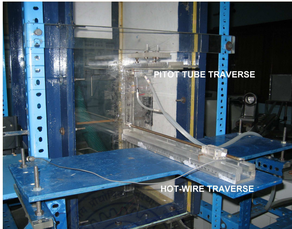
Figure 3.4: Photograph of the pitot tube and Hot-wire traverse.
