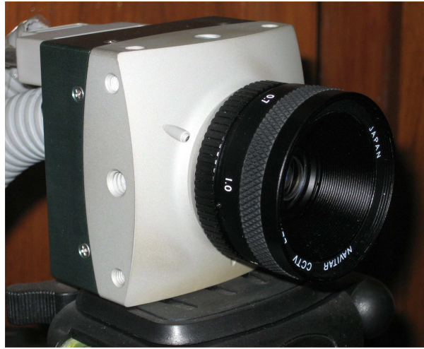
Figure 3.13: Photograph of the high speed CMOS camera used in present experiments.
