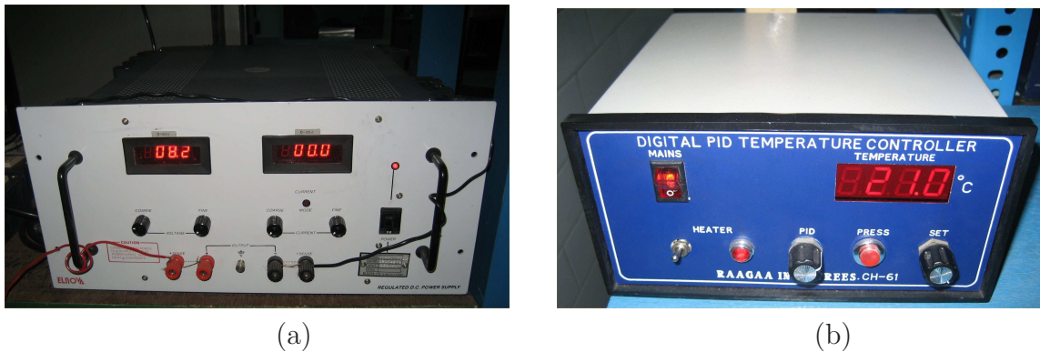
Figure 3.9: Photograph of the (a) Regulated DC Power supply, and (b) Digital PID temperature controller.
