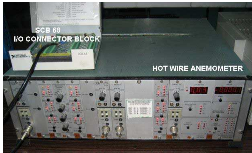
Figure 3.14: Photograph of the Hotwire anemometer used in present experiments.
