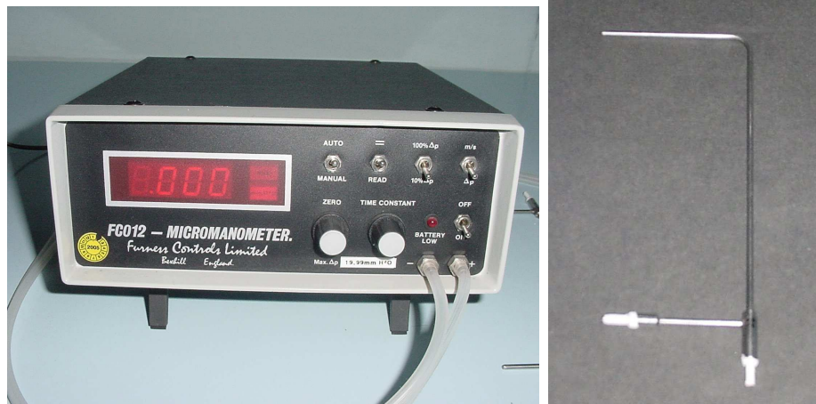
Figure 3.15: Picture of the micromanometer (left) and pitot static tube (right) used during the experiment
