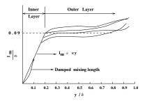
For  $(y/\delta) < 0.2$ ,  $I_m$  is nearly  $\propto y$  with  $\kappa \sim 0.41$ . Very close to the wall, however,  $I_m$  is somewhat lower (damped) than that suggested by  $I_m = \kappa y$ .
