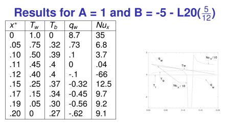
Strange things happen.  $T_w$  reduces to  $T_i = 0$  at  $x^* = 0.2$ .  $T_b$  increases from 0 till  $x^* = 0.11$  but then falls.  $q_w > 0$  for  $x^* \le 0.11$  but then turns negative resulting in negative Nu which then again rises to Nu = 18 at  $x^* = 0.13$  and then again falls. For  $x^* > 0.12$ ,  $T_b > T_w$ .
