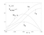
Note that  $Nu_{x,max} = 7.48$  occurs at x/L = 0.5 where  $q_{w,max}$ occurs, but  $T_{w,max}$  and  $T_{b,max}$ occur at x/L = 0.95. This problem is of relevance to Nuclear reactors.
