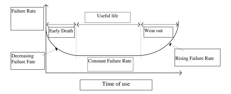
Preventive maintenance is to be done during the product's <u>useful life</u>. This reduces failure rate and also delays the onset of wear out.
