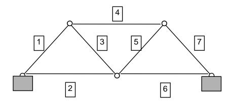
Let the event that element i of the structure fails be denoted by  $F_1$  and let the probability of failure be  $P(F_1)$ . It is assumed that the failure of the different elements is statistically independent, <u>but not</u> mutually exclusive. Also, the structure fails if any element of the structure fails. It is given that
