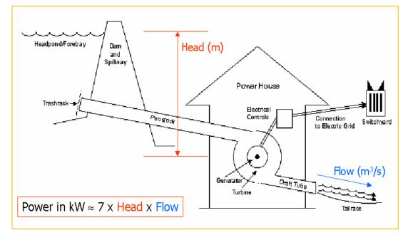
The main components of a hydel power plant are:
